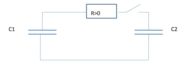
Capacitors are of the same value, 1F; Initially, C1 is charged to V volts, and C2 is in a fully discharged state. The switch s closed at t = 0. Determine the energy dissipated in R at t = infinity
